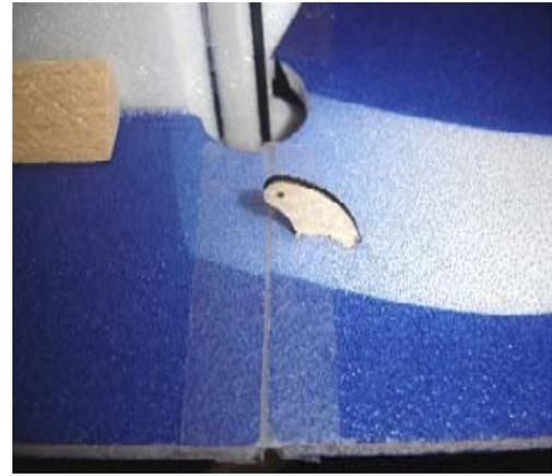
Step 4: Using 5 minute epoxy, glue the firewall assembly to the front of the fuselage. Next, glue the two firewall reinforcement braces behind the firewall on top of the fuselage.
