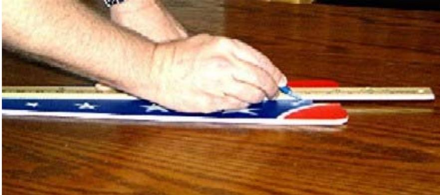
**Step 3a:** Hinge both the ailerons to the wing and the elevator to the horizontal stab using Blenderm hinge tape. When applying the tape to the ailerons and elevator, be sure to check that they deflect as far as they will go, so you have maximum up/down deflection.
