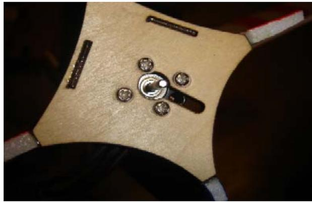
Connect the electronic speed control to the motor and attach it to the fuselage using Velcro. Plug in the three wires from the electronic speed to the motor. Plug the flat connector from the electronic speed control into the micro receiver's throttle position.
