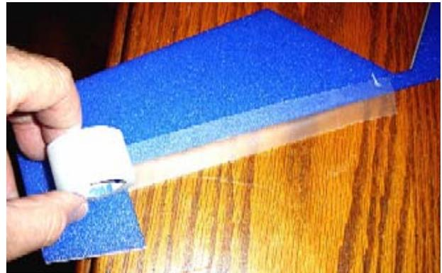
When applying hinge tape to the control surfaces, hinge both sides as shown. The best way to apply the tape is with the hinge line reflexed to one side so the surface is flat when the tape is applied. This way the control surface will move freely either direction without binding.
