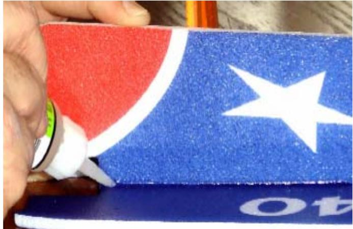
**Step 3c:** Insert the horizontal stab/elevator assembly into the slot in the rear of the fuselage. Measure from the stab tips to the wing tips to make sure the stab is aligned with the wing. Eyeball from the rear to sure the wing and tab line is parallel.
